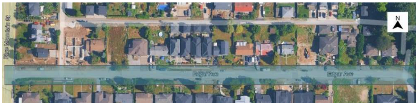
Figure 6.1.5: Edgar Avenue conceptual design catchment area. Road, driveway and future sidewalk implementation contribute to runoff.
