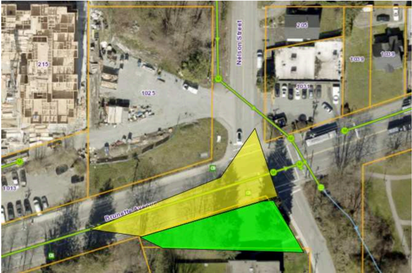
Figure 6.1.6: Mackin Park conceptual design catchment area. Green highlighted areas indicate pervious areas (0.17 acres) and yellow highlighted areas indicate impervious areas (0.17 acres).
