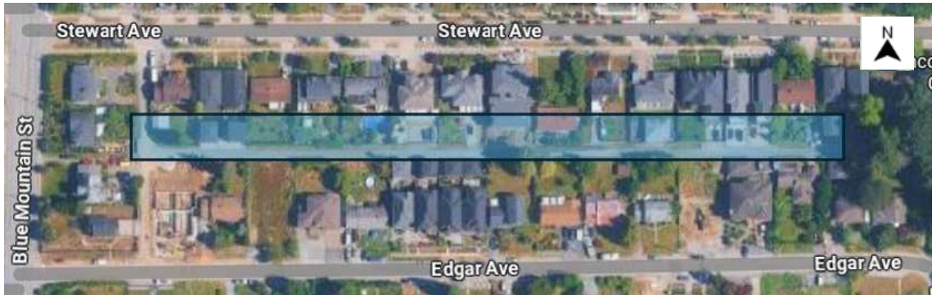
Figure 6.1.4: Edgar Laneway conceptual design catchment area. Homes on the lot include roof gutter lines directly connected to the storm sewer system, and therefore do not contribute to the pavers. Greater impervious contribution is anticipated by post-development driveways and any fugitive runoff.
