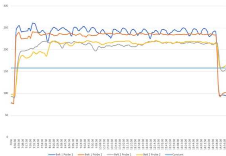
Figure 10: Belt press probe testing to monitor temperature above 158°F (Merrell 2019).
