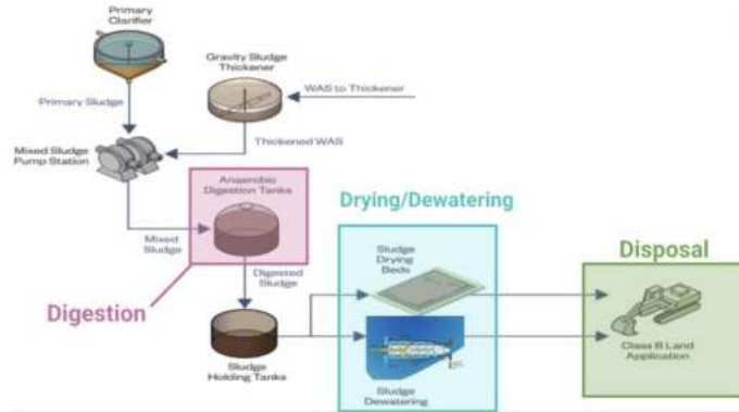
Figure A 1. Process flow diagram of HFC AWTP (SustainaCore, 2025).
